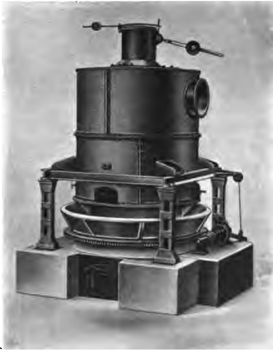
FIG. 50.—External View of "Hilger" Gas Producer.
